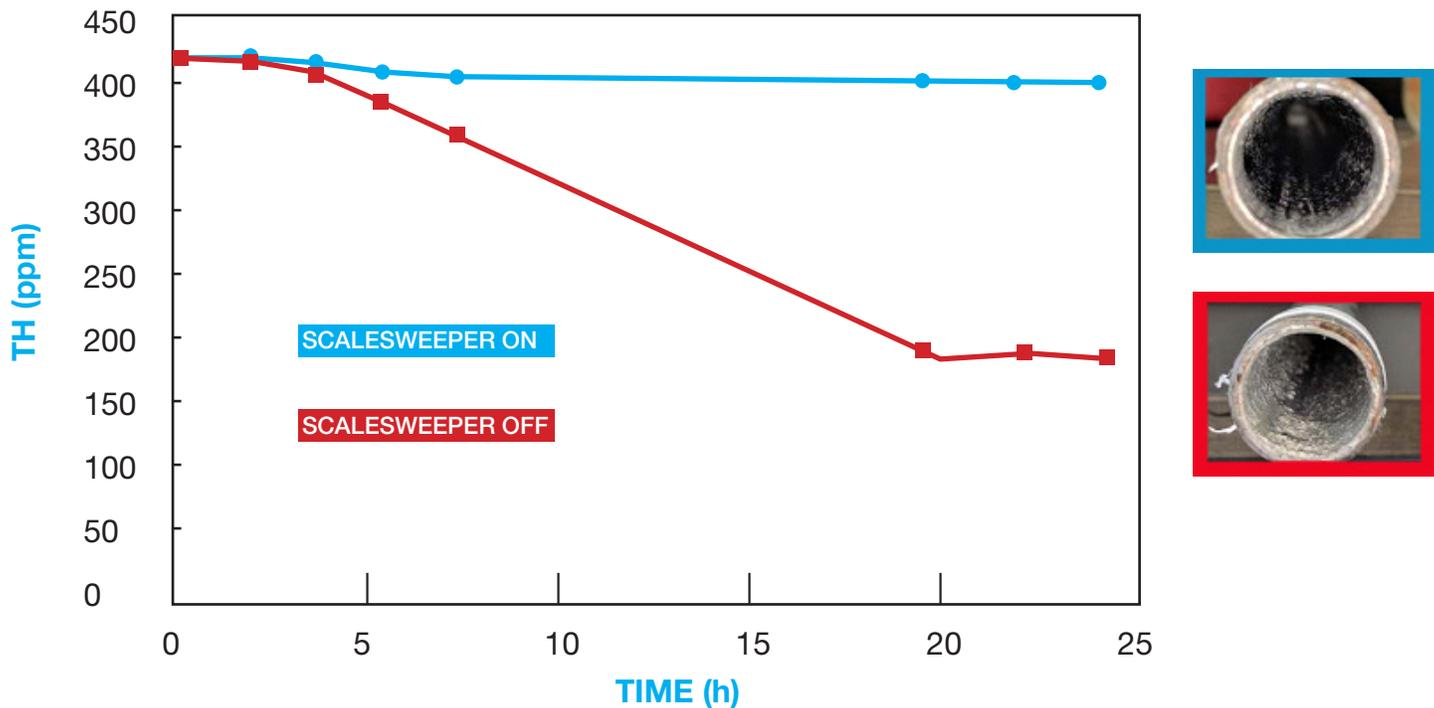
**Note on Figure 1:** Two 24-hour tests were conducted to prove Scalesweeper’s effectiveness in reducing scale formation in pipe systems. With **Scalesweeper turned off** (the red line) shows total hardness measured in the recirculated water reduces dramatically. This is due to hard scale coming out of the water and attaching to the pipes as pictured. With **Scalesweeper turned on** (the blue line) shows no change in hardness as the scale is not forming on the pipe as shown in photo.
